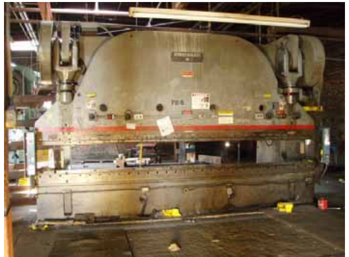
Press Brake, Cincinnati 13, s/n 37054, 12', 400 ton
